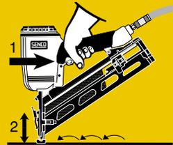
● With a "Restrictive" trigger, nails can only be driven one way. First depress safety element against work surface then pull trigger. This feature is helpful when precise fastener placement is required.
