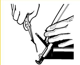
● Remove jammed fastener. Close door and latch.
