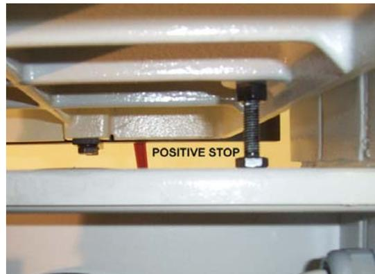
**Fig 27 POSITIVE STOP BOLT**
