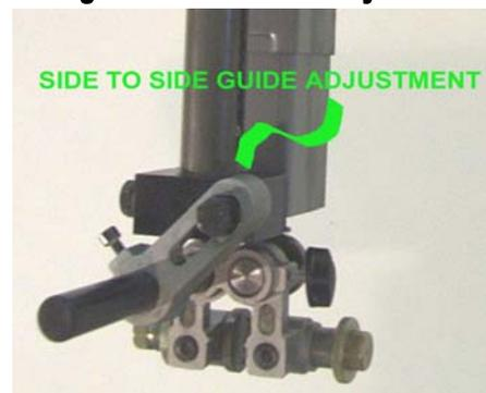
**Fig 15 Horizontal Adjustment**
