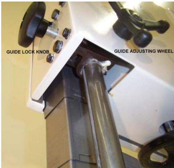
**Fig 22 Guide Post Adjustment**
