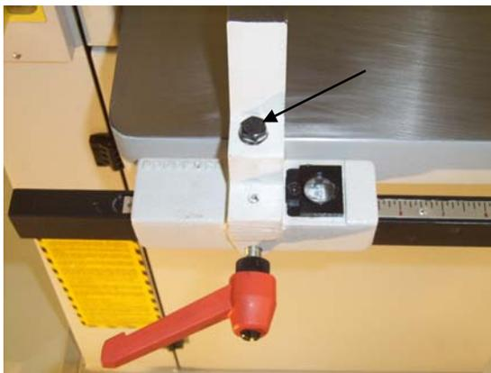
Blade drift means the blade isn't cutting parallel to the fence. Every blade will cut in a slightly different manner and you may have to adjust the fence angle to compensate for this drift. To check blade drift, mark a straight line on a board 24" long, rip the board freehand while carefully following the line. About halfway, through the cut, stop the saw and leave the board in place. Mark the side of the board on the saw table with a soft pencil. This line indicates the
