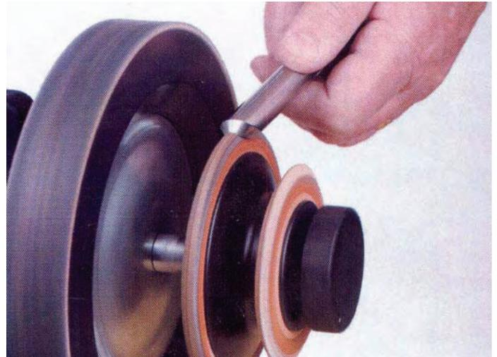
**Hone the flute of the tool on the profiled leather honing wheel as shown. I recommend another light pass on the grinding wheel after this honing.**
