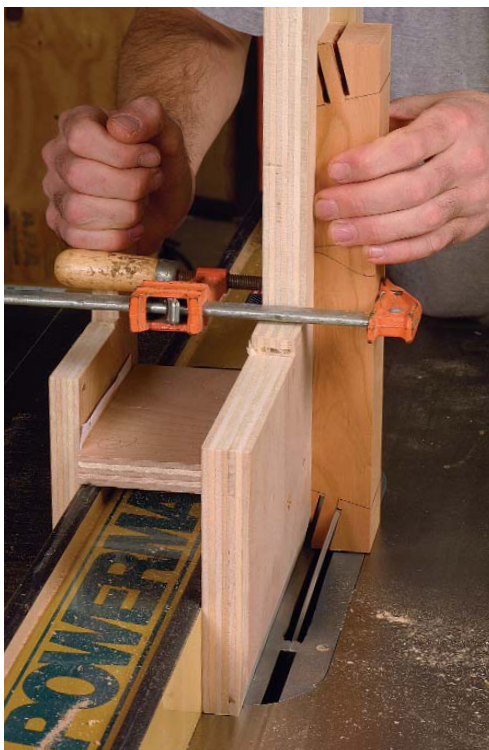
Cut the tenons on the rails while the stock is square. Make the cheek cuts first (left), then make the shoulder cuts (above).
