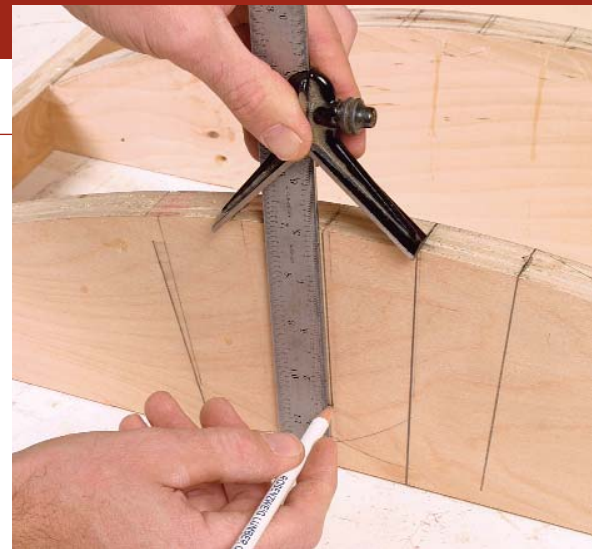
Figure out sections and angles right on the form. Use a center divider to draw lines straight down from each division.
