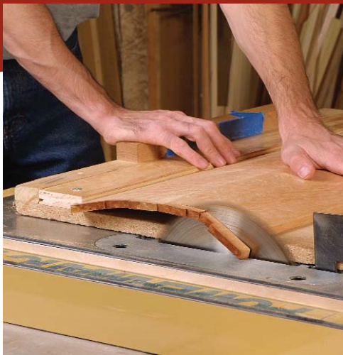
With the concave side down, trim the panel to size. Use a sled for crosscutting, with the blade at its highest point.
