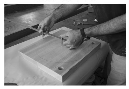
Around & around. Here I'm marking out the diameter of the seat. Note the two holes in the corners of the blank. These are test mortises that will allow me to test the fit of the tenons on the legs. Waste not, blah blah, blah.
