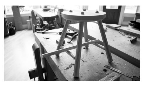
Stretchers. The side stretchers are installed. And the medial stretcher is laid on top. Now we're ready to drill the mortises for the medial stretcher.
