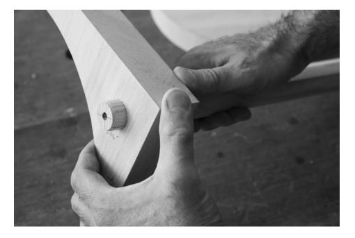
Test each tenon. After I cut each tenon, I check it in the test mortise (made with scraps from the seat). This is a backstop because I don't trust my bedan sizing tool, though it has yet to let me down.
