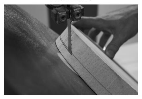
Around again. After cutting the seat round, tilt the saw's table to 45° to cut the bevel on the underside of the seat. Mark the 1/2" bevel on the seat's edge and follow that with your saw's blade.
