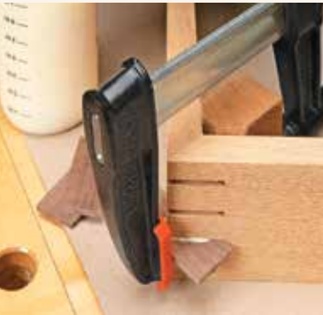
▲ The corner block makes it possible to clamp the splines in position.
