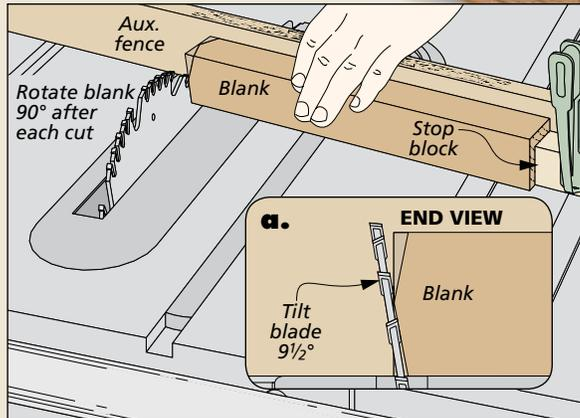
**Front Caps.** To make the front mortise caps, cut four  $9\frac{1}{2}^\circ$  bevels on the end of a long blank. Use a stop block to ensure the beveled faces meet at the center.
