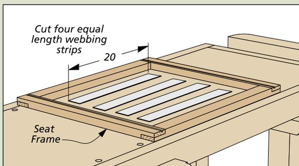
**Webbing.** The elastic chair webbing will be stretched slightly to fit the frame. So I cut four equal pieces about 3" less than the distance between the kerfs.
