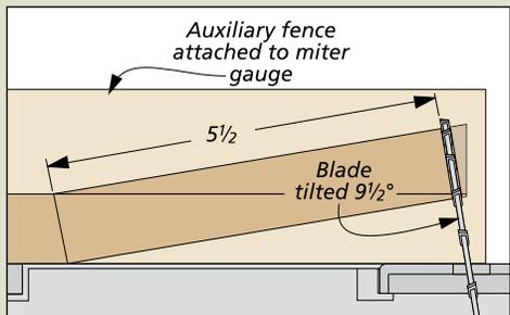
**Square the End.** Finally, you can take the blanks to the table saw to square the ends. You'll need to tilt the saw blade  $9\frac{1}{2}^\circ$ .
