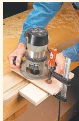
▲ This simple jig makes routing the groove on the underside of the bent arm smooth sailing.
