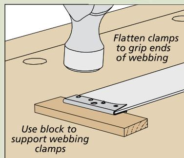
**Clamps.** Next, a webbing clamp is "pinched" tightly over each end of the webbing strips.
