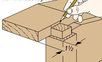
**In Position.** The tenons are used to mark the location of the mortises on the sides of the arms.
