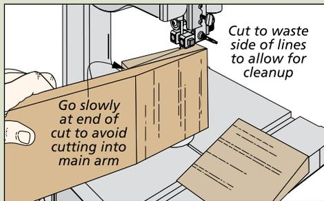
**Cut & Clean.** After carefully removing the waste at the band saw, I cleaned up the two faces with a block plane and sandpaper.
