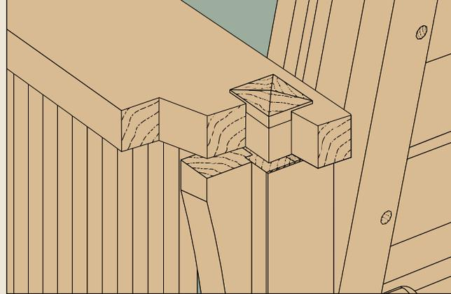
The sloping, “bent” arms of the chair add a few challenges. The first is the angled tenon on the top of the back legs that matches the “fall” of the arms. It just takes a step-by-step approach to get the job done.
