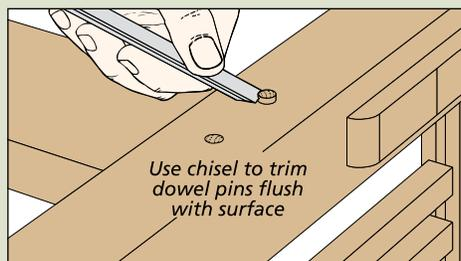
**Trim Them Flush.** When the glue is dry, you can use a chisel, bevel down, to carefully trim the dowel pins flush to the surface.
