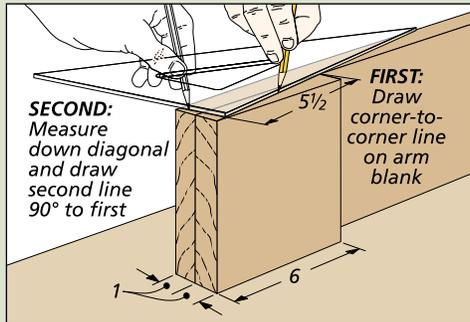
**The Lower Side.** First, lay out the lower side of the bend by simply drawing a corner-to-corner line on the short lower arm block.
