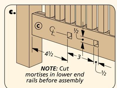
lower rails (detail 'c' on previous page). These mortises are for the stretchers that add some stiffness to the frame.
