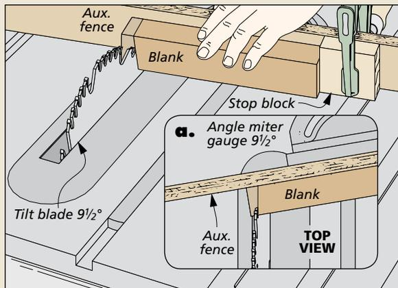
**Back Mortise Caps.** Start by clamping a stop block to the miter gauge. Then make a compound bevel cut — with both the blade and miter gauge angled  $9\frac{1}{2}^\circ$ .
