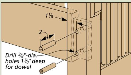
**Drill & Insert.** After drilling holes for the dowel pins, cut them to rough length and “ease” one end before driving them in.
