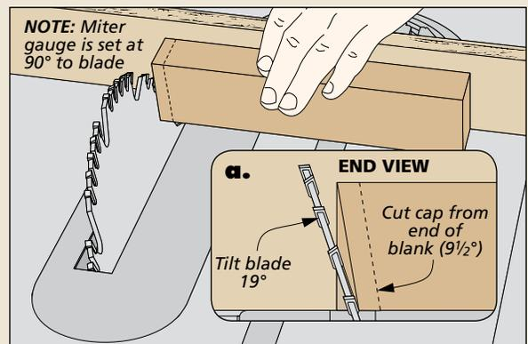
**Fourth Cut.** To cut the final face, tilt the blade  $19^\circ$  and sneak up on the cut until the four beveled faces meet at a point centered on the end of the blank.
