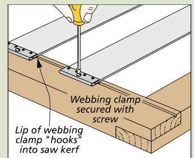
**Kerf.** After fastening one end, stretch the strip to fit to the opposite kerf and screw it down.
