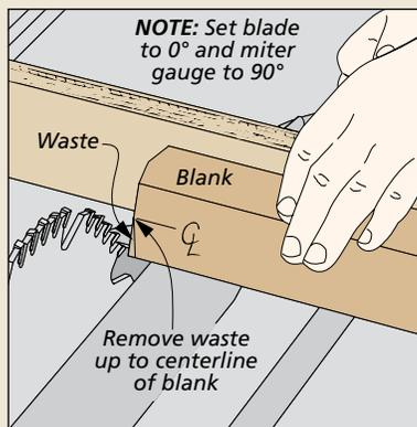
**Third Cut.** With the miter gauge square to the blade and the blade at  $0^\circ$ , sneak up on the third face.
