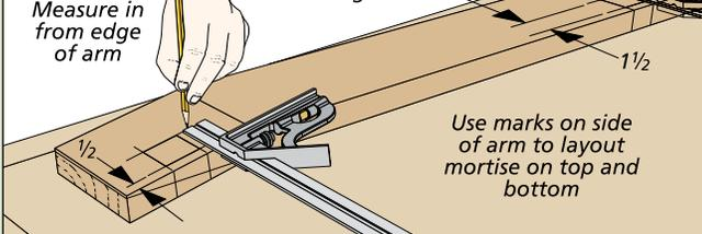
**Mortise Layout.** The marks on the side of the arms can then be squared to the top and bottom to give you the right spacing. Keep in mind that the rear mortise is cut at an angle.
