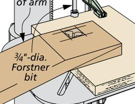
**Drill Press.** Next, the mortises are started by drilling out the waste. Be sure to use a backup piece. You'll have to angle the table for the rear mortises.
