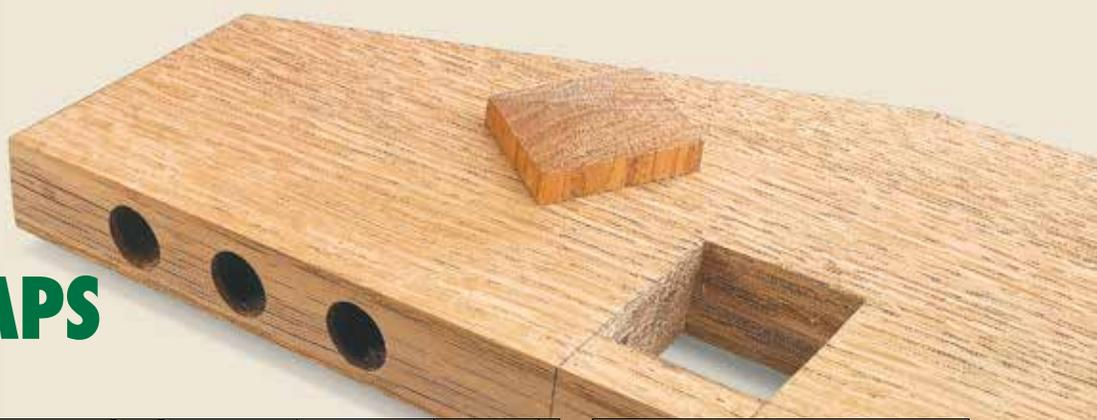
One of the details of the Morris chair that I really like are the beveled caps that fit into the leg mortises in the arms of the chair. The top of each cap has four beveled faces that meet at the center, resembling a flattened-out pyramid (see photo).
