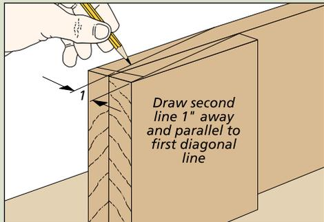
**The Upper Side.** Next, measure up 1" from your first line and draw a second line. This line will be the top side of the bend.
