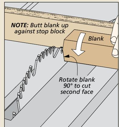
**Second Cut.** Without changing the setup, rotate the blank  $90^\circ$  to make the second cut.
