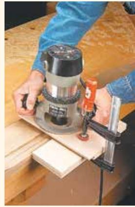
▲ This simple jig makes routing the groove on the underside of the bent arm smooth sailing.
