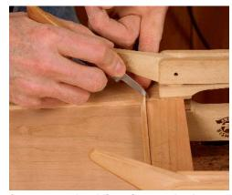
**Quarter-round molding trims out the door.** The molding is shaped on the router, then mitered to fit the door. Becksvoort simply glues the molding to the rails and the stiles.
