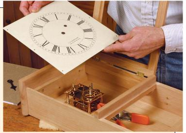
Align the movement with the face. With the movement roughly centered inside the clock, lay the face in place and make adjustments until the hands are properly centered. Use an awl to make screw holes through the movement.
