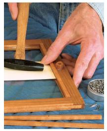
**Securing the glass.** After setting the glass into the rabbet, small glass supports are nailed into place.
