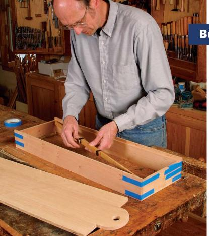
**Quick clamps for temporary strength.** The false top and false bottom are simply butt-joined and glued to the sides. The actual top and bottom will reinforce this joint. Before the glue sets, check to make sure the case is level and square.
