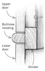
Bullnose molding separates top and bottom doors. Shape the profile using a roundover bit, then cut it to fit flush with the sides.
