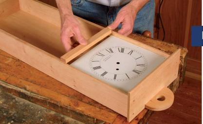
**Horizontal divider catches the doors.** The horizontal divider is sized to act as a doorstop for both doors. It is set into the stopped rabbet that holds the clock face.
