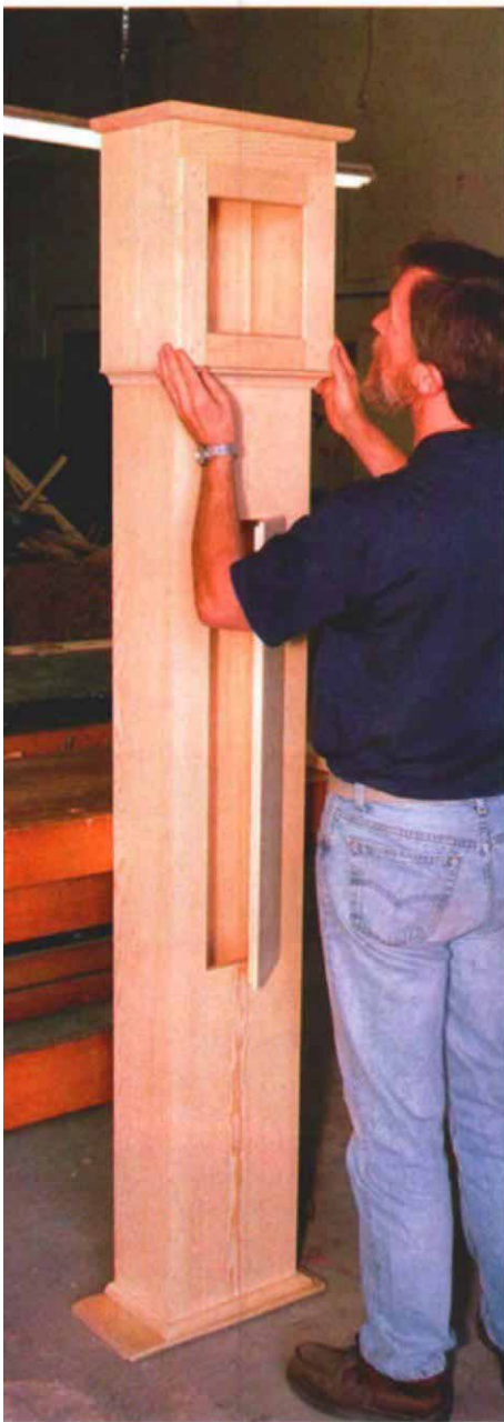
Slide-on bonnet—The bonnet for this Shaker tall clock rests on transitional molding at the top of the case. It slides on and off to provide access to the clock's movement.
