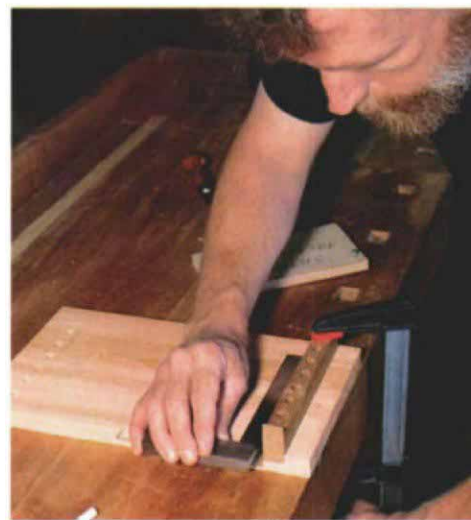
Flip jig, and drill bottom. The jig, with its fence removed, is flipped over and aligned with layout lines on the case bottom to drill matching holes.
