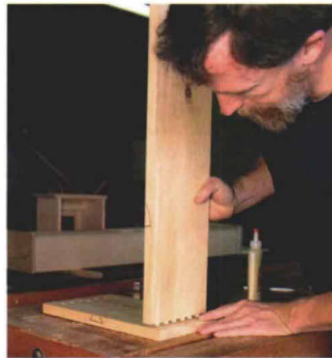
Test-fit. The jig ensures that dowels line up correctly, even if guide holes are not perfectly spaced or centered.
