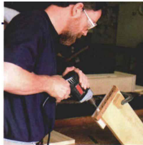
Doweling jig —Holes bored in a hardwood scrap guide the bit as the author drills out a case side for glue dowels.
